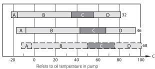
E.g. Hydraulic oil 32: The designation "32" denotes the viscosity is 32 cSt at 40 °C. Lowest start temperature is -23 °C and highest working temperature 82 °C. Ideal working temperature is 35 - 55 °C.
