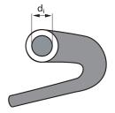
If the suction line is more than 2 m long the internal diameter must be increased by 10 mm for each meter extension.
