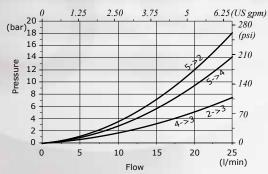
Pressure compensator (inlet to work port - spool 42 type)
