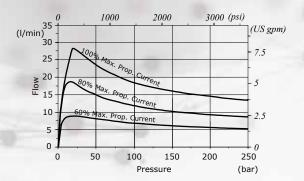
Flow vs. current (with 10,5 bar/152 psi inline compensator - spool 42 type)
