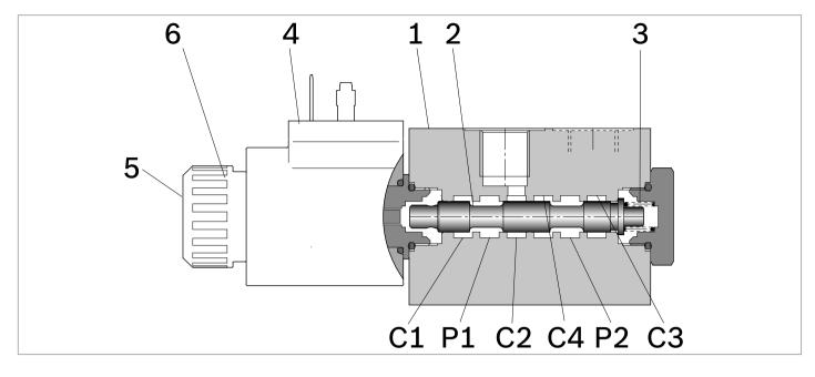
A valve basically consists of a housing (1), a control spool (2), a return spring (3) and a solenoid (4). It is designed to connect two inlet lines **P1** – **P2** (normally a set of hoses) and divert them to either the outlet ports (**C1** – **C4**) with spool in position "0", when the solenoid is de-energized, or to the outlet ports (**C2** – **C3**) with spool in position "1", when the solenoid is energized.
