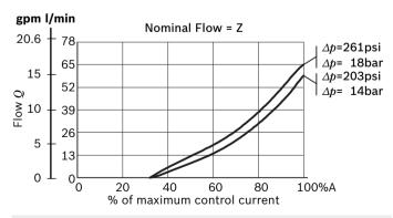
The curves refer to the spool fully open. Measured with hydraulic fluid ISO-VG32 at 45° ±5 °C (113° ±9 °F); ambient temperature 20 °C (68 °F).
