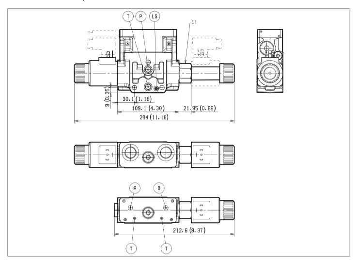
1 Flow-boost system only for spool with nominal flow 9 and Z. It always mounted on "b" side of the valve.
