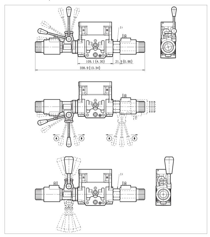
**1** Flow-boost system only for spool with nominal flow 9 and Z. It always mounted on the opposite side of the lever manual override.
