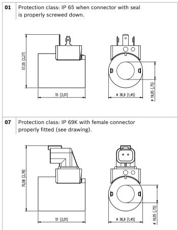
12 **EDG-DP...** | 4/3 and 4/2 Proportional directional valve elements Electric connection
