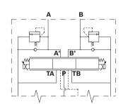
**= M0** (Relief valve with anticavitation option)
