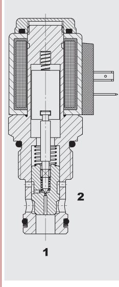
The directional valve is a pilot operated valve in poppet style.
