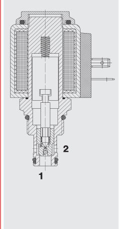
The directional valve is a pilot-operated valve in a poppet design.
