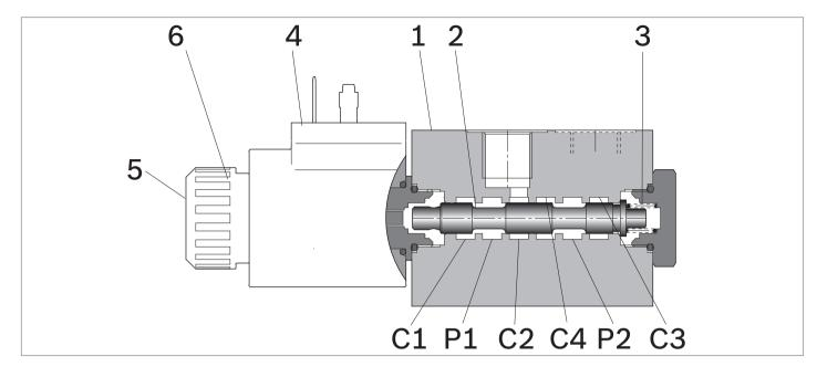
A valve basically consists of a housing (1), a control spool (2), a return spring (3) and a solenoid (4). It is designed to connect two inlet lines P1 - P2 (normally a set of hoses) and divert them to either the outlet ports (C1 - C4) with spool in position "0", when the solenoid is de-energized, or to the outlet ports (C2 - C3) with spool in position "1", when the solenoid is energized.
