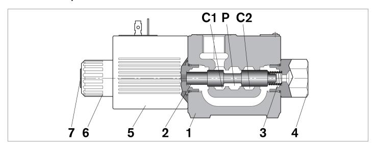
A valve basically consists of a housing (1), a control spool (2), a return spring (3) and a solenoid (5). It is designed to select which one of two circuits (C1 or C2) is to be supplied with the oil delivered from one single hose (P): with spool in position "0", when the solenoid is de-energized, the flow goes from P to C1, with spool in position "1", when the solenoid is energized the flow goes from P to C2.
